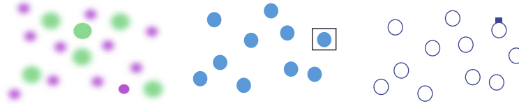
Figure 5.13 A number of highlighting methods that use positive asymmetric preattentive cues: sharpness, added surrounding feature, added shape.
